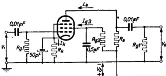
$$R_a = 0,22 \text{ M}\Omega; \quad R_{g1} = 1 \text{ M}\Omega; \quad R_{g1'} = 0,68 \text{ M}\Omega.$$
