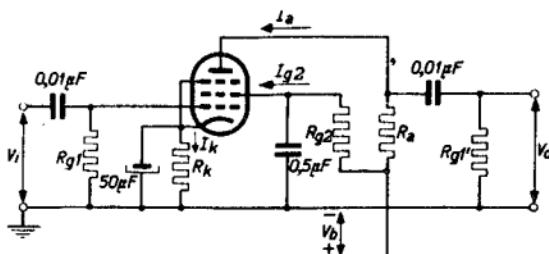
$$R_a = 0,22 \text{ M}\Omega; \quad R_{g1} = 1 \text{ M}\Omega; \quad R_{g1}' = 0,68 \text{ M}\Omega.$$
