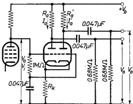
Va should be adjusted to the specified value of  $I_a + I_a'$
