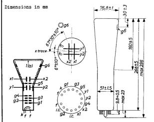
The post-deflection acceleration helix is connected between g6 and the isolation shield g5.
