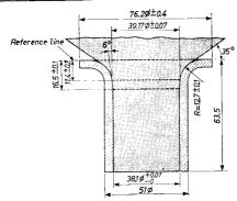
The reference line is determined by the plane of the upper edge of the gauge when it is resting on the come. The inner surface of the coils should not extend into the shaded region.
