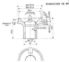
REFERENCE LINE GAUGE. The reference line of the tube 1s determined by the plane of the upper edge of the flange of the gauge when it is resting on the cone.
