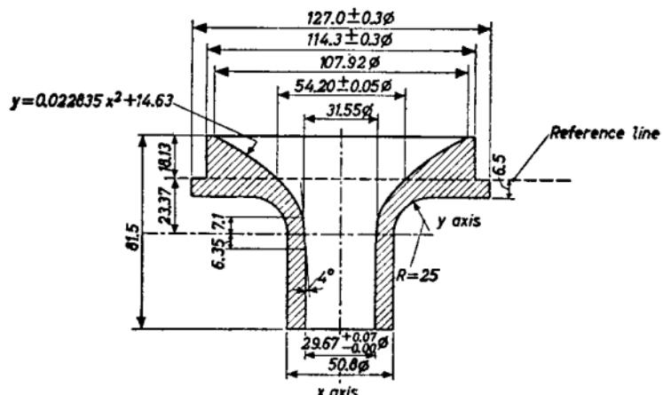
If x and y are expressed in inches, the parabolic formula for the inner contour reads  $y = 0.58 x^2 + 0.576$
