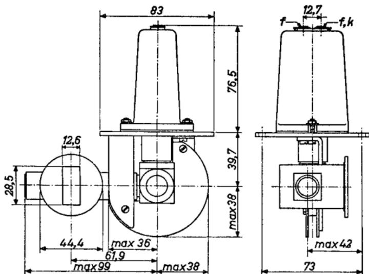
Magnetron output Designed for coupling to standard rectangular waveguide RG-51/U. For drawing of this waveguide see front of this section
