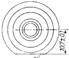
1) Max. eccentricity of the axis of the radiator core cap or the grid terminal flange with respect to the axis of the cathode terminal is 0,38 mm.
