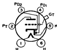
The 75 is a heater type of tube consisting of two diodes and a high-mu triode in a single bulb. It is for use as a combined detector, amplifier, and automatic-volume-control tube in
