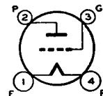
The 71-A is a power-amplifier tube of low-output impedance for use in the output stage of audio-frequency amplifiers.
