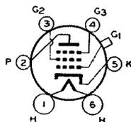
The 6C6 is a triple-grid tube of the heater-cathode type recommended for service as a biased detector in radio receivers designed for its characteristics. This tube is capable of delivering a large audio-frequency output voltage with relatively small input voltage. Significant among its electrical features are its sharp plate current "cut-off" with respect to grid voltage. The 6C6 is constructed with an internal shield connected to the cathode within the tube.
