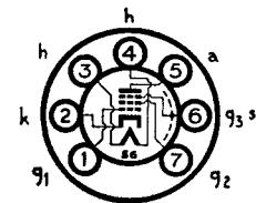
The BRIMAR 6AM6 is an indirectly heated high slope R.F. pentode suitable for a wide variety of applications. It may be used as an R.F., I.F. or video amplifier, as a limiter, or as a frequency changer at frequencies up to 100 Mc/s in conjunction with a suitable oscillator.
