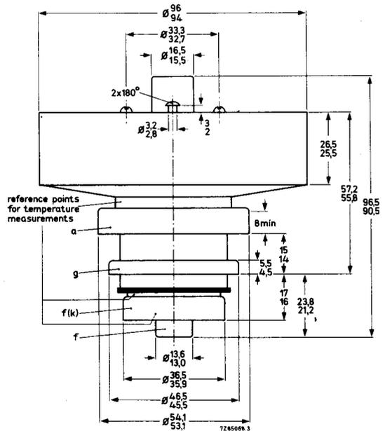
The radiator and the terminals are situated within concentric cylinders of the following dimensions:
