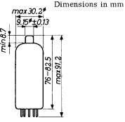
Pins 1, 5 and 9 may be used to connect an anti-corona ring.
