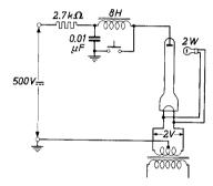
The minimum value if  $V_{\mbox{ign}}$  is only valid if some ambient illumination is present. Hence in darkness the presence of a small light-source (about 2W) is necessary.
