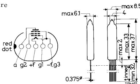
Leads should not be soldered nearer than 5 mm to the seal
