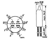
Connections should not be soldered nearer than 5 mm to the seal. Leads should not be bent nearer than 1.5 mm to the seal.
