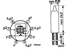
Leads should not be soldered nearer than 5 mm to the seal Leads should not be bent nearer than 2 mm to the seal
