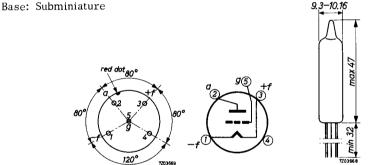
Directly soldered connections to the leads of this tube must be at least 13 mm from the seal and any bending of the leads must be at least 1.5 mm from the seals.
