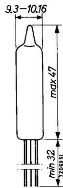
Directly soldered connections to the leads of this tube must be at least 13 mm from the seal and any bending of the leads must be at least 1.5 mm from the seal.
