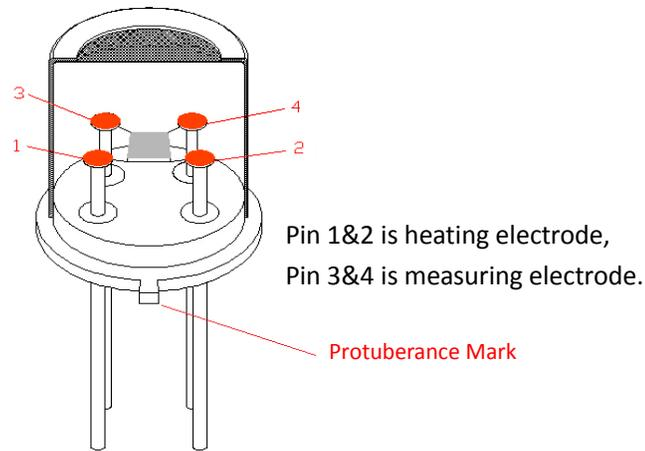
**Fig8.Pin Schematic Diagram**
