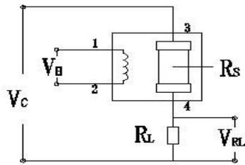
This circuit shows the basic measuring circuit of sensor. Two voltage should be applied to this sensor, heating voltage ( $V_H$ ) and circuit voltage( $V_C$ ).  $V_H$  is used for supplying a certain temperature which can be DC or AC.  $V_{RL}$  the voltage on the load resistance( $R_L$ ) which connects to the sensor in series.  $V_C$  is supply the test voltage for  $R_L$  and it must be DC.
