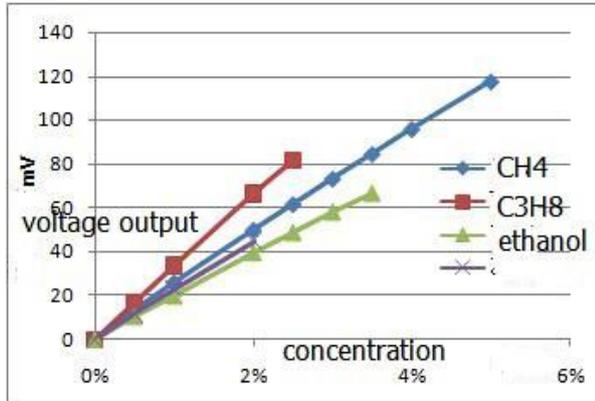
**Fig3. Sensitivity Curve**
