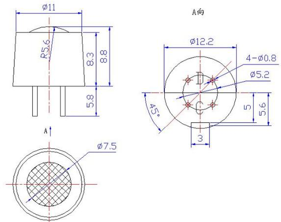
Fig1. Sensor Structure
