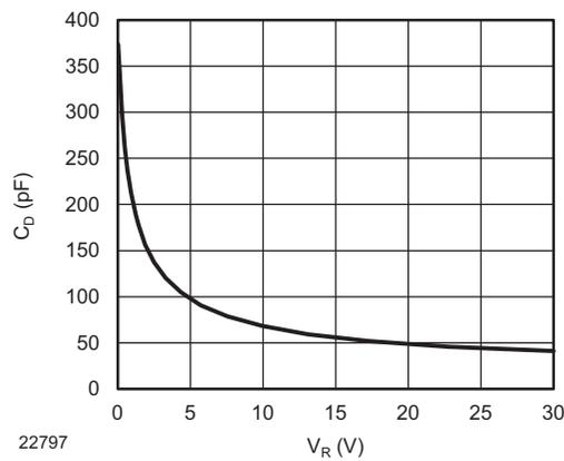
Fig. 3 - Typical Capacitance vs. Reverse Voltage
