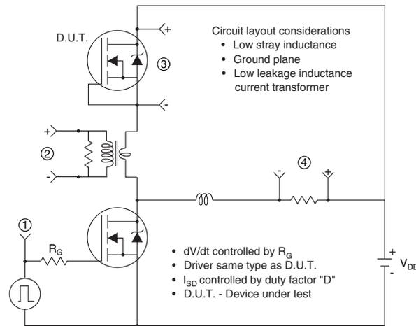
Fig. 18 - Peak Diode Recovery  $dv/dt$  Test Circuit
