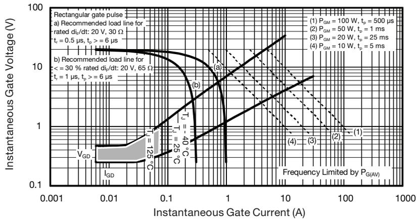
Fig. 8 - Gate Characteristics
