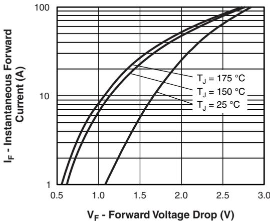
Fig. 1 - Typical Forward Voltage Drop Characteristics
