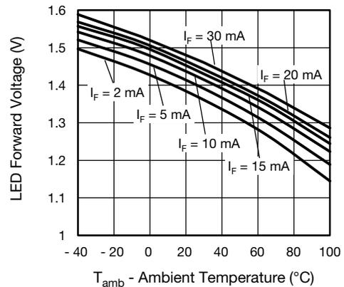
Fig. 6 - LED Forward Voltage vs. Ambient Temperature
