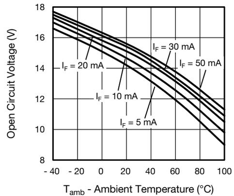
Fig. 5 - Open Circuit Voltage vs. Ambient Temperature
