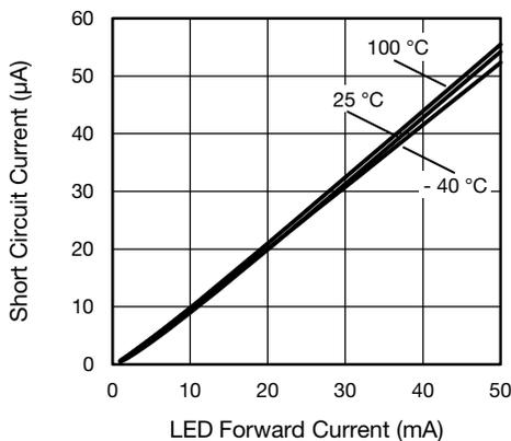
Fig. 3 - Short Circuit Current vs. LED Forward Current
