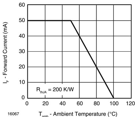
Fig. 1 - Max. Permissible Forward Current vs. Ambient Temperature
