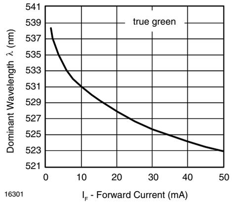
Fig. 10 - Dominant Wavelength vs. Forward Current
