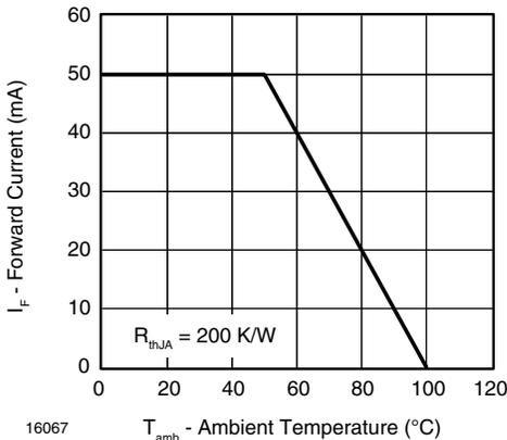
Fig. 1 - Forward Current vs. Ambient Temperature for InGaN
