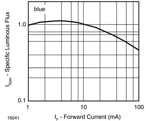
Fig. 6 - Specific Luminous Flux vs. Forward Current
