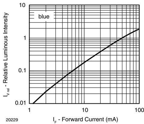
Fig. 5 - Relative Luminous Flux vs. Forward Current
