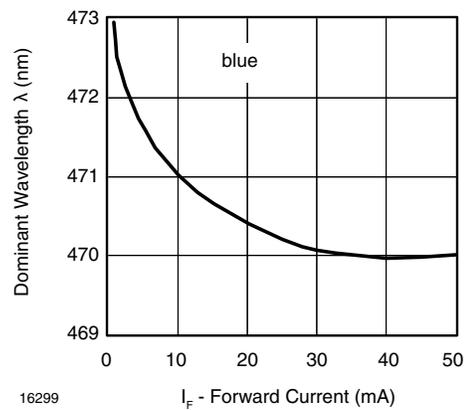
Fig. 8 - Dominant Wavelength vs. Forward Current
