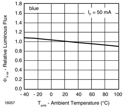
Fig. 7 - Rel. Luminous Flux vs. Ambient Temperature
