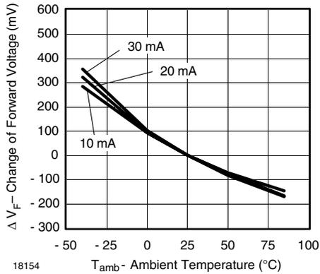
Figure 7. Change of Forward Voltage vs. Ambient Temperature
