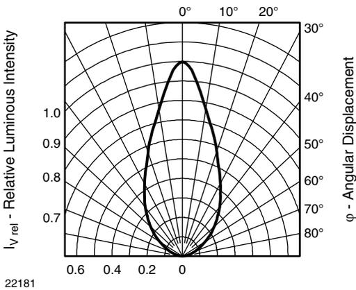
Fig. 2 - Relative Luminous Intensity vs. Angular Displacement
