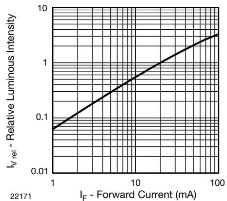
Fig. 5 - Relative Luminous Intensity vs. Forward Current
