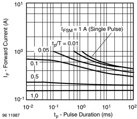
Fig. 3 - Pulse Forward Current vs. Pulse Duration
