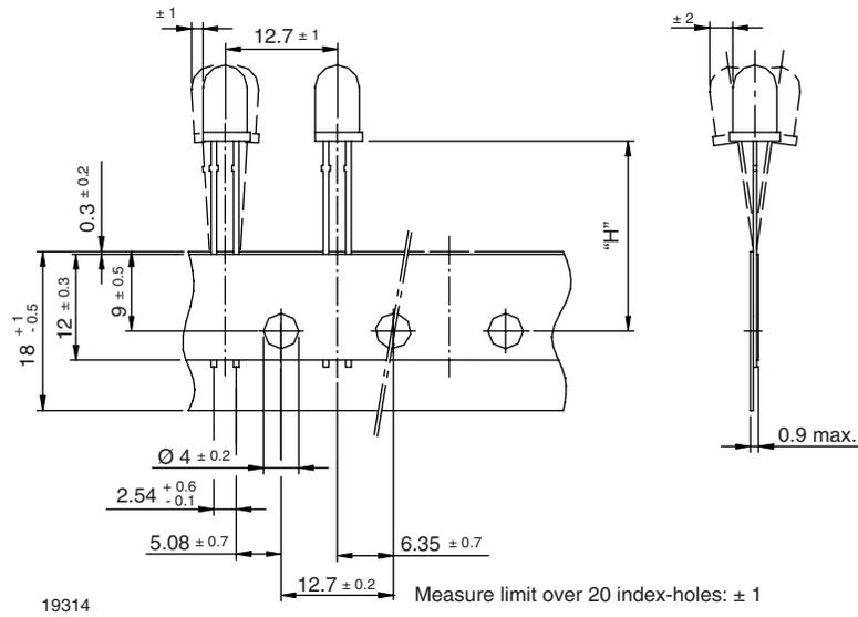
Fig. 10 - Ø 5 mm Devices on Tape
