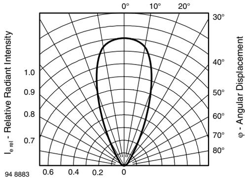
Fig. 9 - Relative Radiant Intensity vs. Angular Displacement
