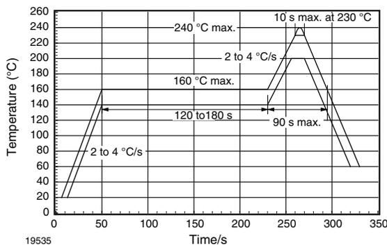
Fig. 3 - Recommended Solder Profile for Sn/Pb soldering
