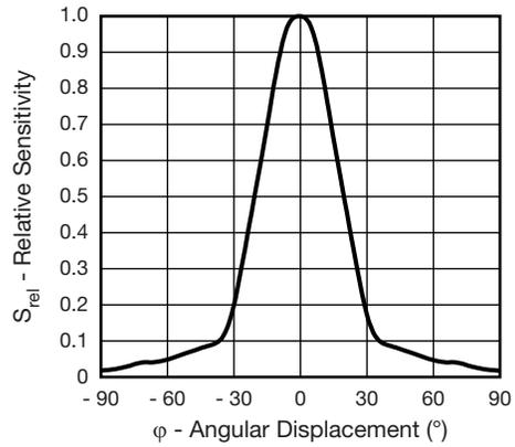
Fig. 6 - Relative Radiant Intensity vs. Angular Displacement
