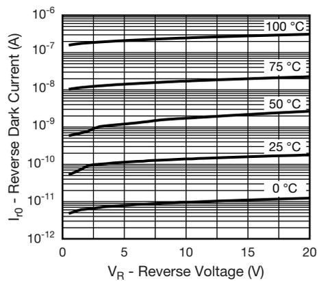
Fig. 7 - Dark Current vs. Reverse Voltage
