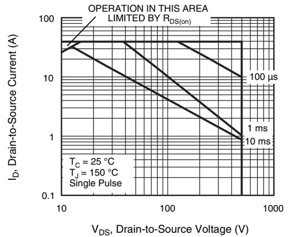
Fig. 8 - Maximum Safe Operating Area (TO-220AB, D<sup>2</sup>PAK)
