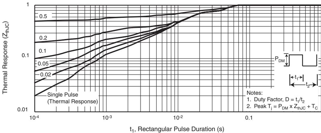
Fig. 11 - Maximum Effective Transient Thermal Impedance, Junction-to-Case (TO-220AB, D<sup>2</sup>PAK)
