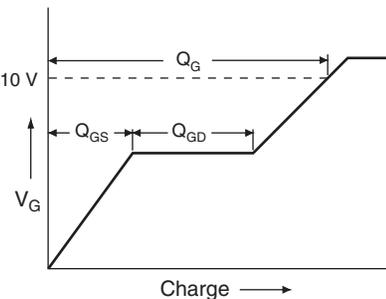
Fig. 17 - Basic Gate Charge Waveform
