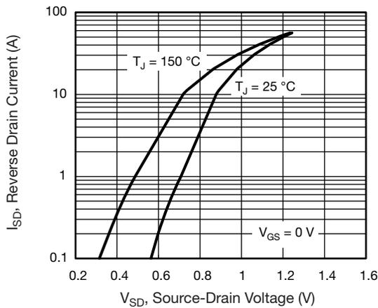
Fig. 8 - Typical Source-Drain Diode Forward Voltage
