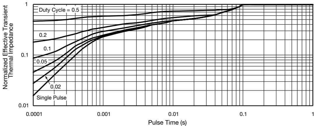
Fig. 12 - Normalized Thermal Transient Impedance, Junction-to-Case
