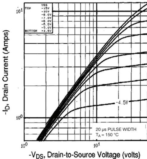
Fig. 2 - Typical Output Characteristics,  $T_A = 150\text{ }^\circ\text{C}$
