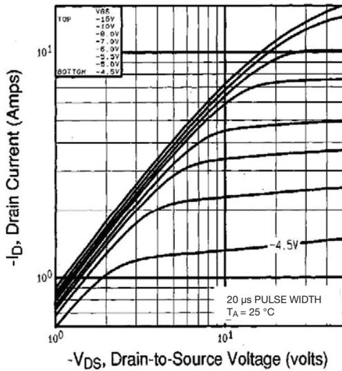
Fig. 1 - Typical Output Characteristics,  $T_A = 25\text{ }^\circ\text{C}$
