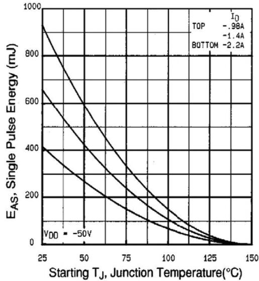
Fig. 12c - Maximum Avalanche Energy vs. Drain Current
