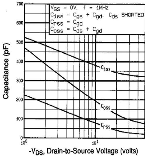
Fig. 5 - Typical Capacitance vs. Drain-to-Source Voltage
