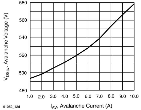
Fig. 12d - Typical Drain-to-Source Voltage vs. Avalanche Current
