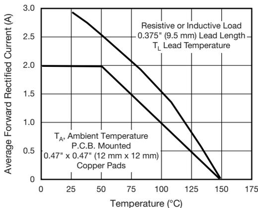
Fig. 1 - Maximum Forward Current Derating Curves
