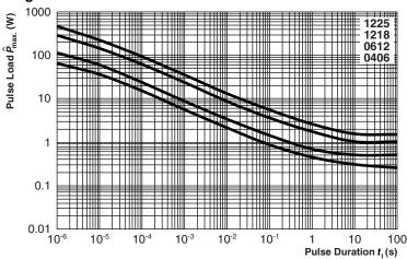
Maximum pulse load, single pulse; applicable if  $\bar{P} \longrightarrow 0$  and n < 1000 and  $\hat{U} \le \hat{U}_{max}$ ; for permissible resistance change equivalent to 8000 h operation
