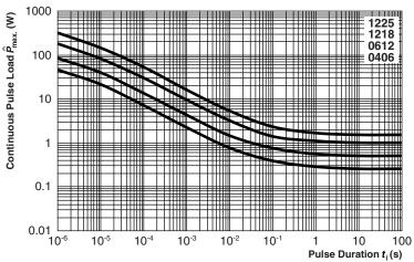
Maximum pulse load, continuous pulses; applicable if  $\vec{P} \leq P$  ( $\vartheta_{amb}$ ) and  $\hat{U} \leq \hat{U}_{max}$ ; for permissible resistance change equivalent to 8000 h operation
