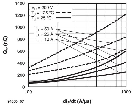
Fig. 7 - Typical Stored Charge vs.  $di_F/dt$
