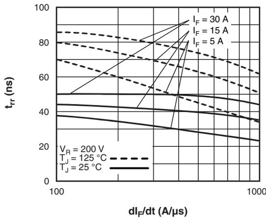
Fig. 5 - Typical Reverse Recovery Time vs.  $di_F/dt$
