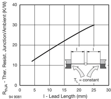
Fig. 1 - Typ. Thermal Resistance vs. Lead Length
