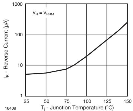
Fig. 4 - Reverse Current vs. Junction Temperature
