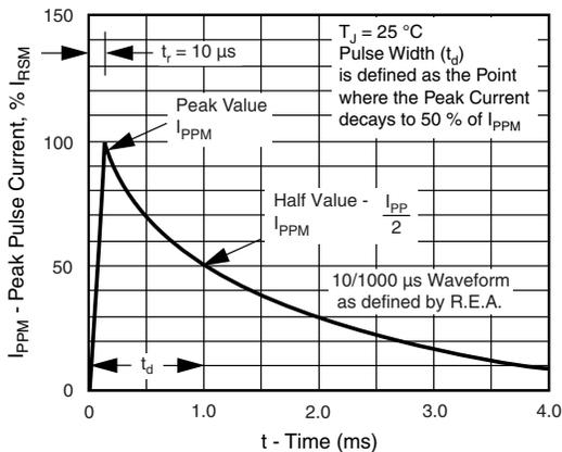
Fig. 3 - Pulse Waveform
