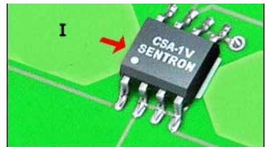
Figure 2 – Sensing current in a PCB trace
