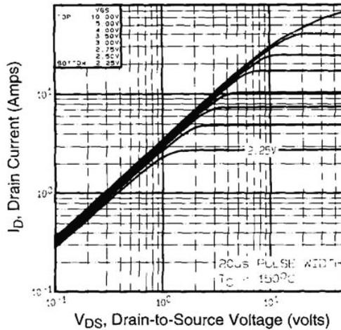
Fig. 2 - Typical Output Characteristics,  $T_C = 150\text{ }^\circ\text{C}$
