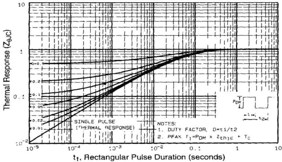
Fig. 11 - Maximum Effective Transient Thermal Impedance, Junction-to-Case
