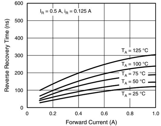
Figure 6. Reverse Recovery Time vs. Forward Current
