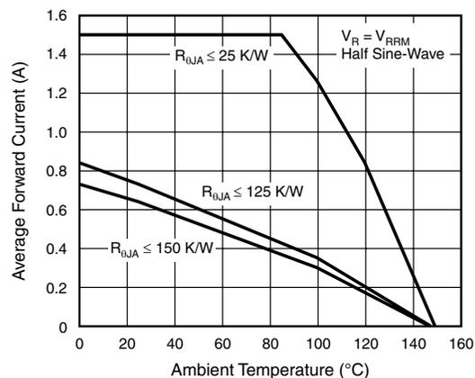
Figure 2. Max. Average Forward Current vs. Ambient Temperature
