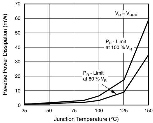
Figure 4. Max. Reverse Power Dissipation vs. Junction Temperature
