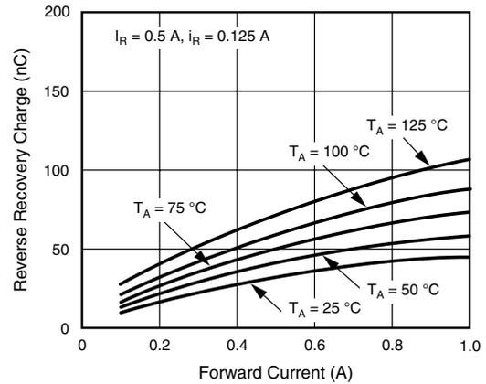
Figure 7. Reverse Recovery Charge vs. Forward Current
