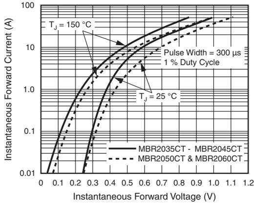
Figure 3. Typical Instantaneous Forward Characteristics Per Diode
