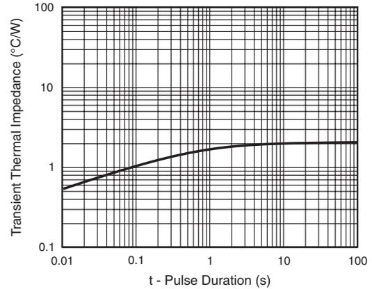
Figure 6. Typical Transient Thermal Impedance Per Diode
