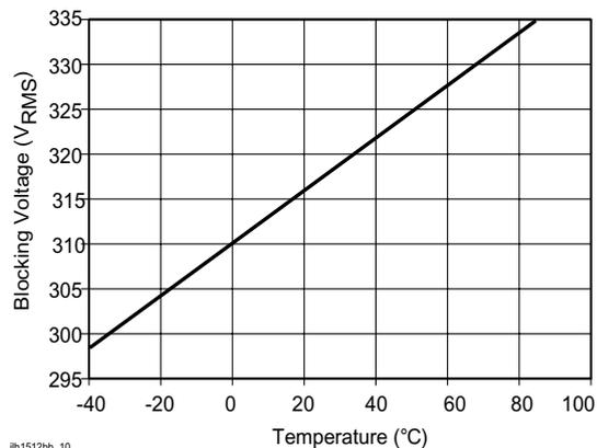
Figure 10. Form B\_Typical Blocking Voltage vs. Temperature
