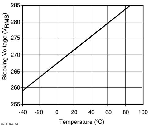
Figure 7. Form A\_Typical Blocking Voltage vs. Temperature
