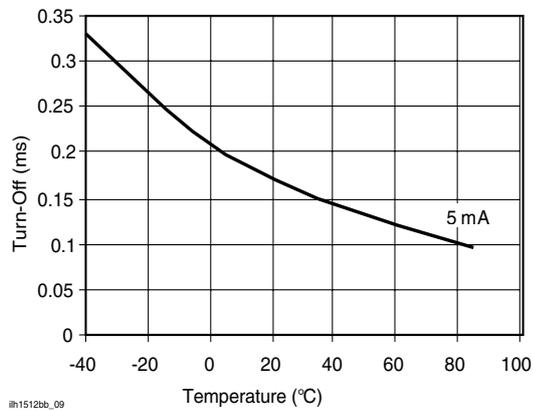
Figure 9. Form A\_Typical Turn-Off vs. Temperature
