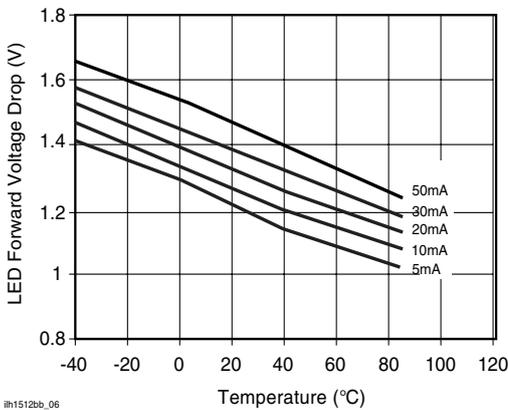
Figure 6. Typical LED Forward Voltage Drop vs. Temperature
